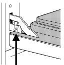
Lock engaged for door removal
